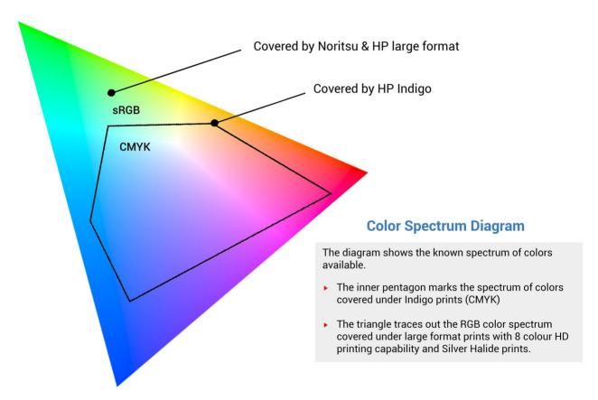
Our HP Indigo 7900 Press has two more primary inks added to the standard CMYK. This will expand the color spectrum that can be printed and results in better color production.
